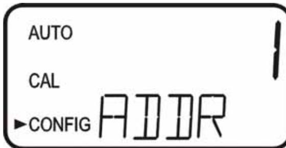
Select the operating mode either ASCII or RTU using the **▲** or **▼** buttons. Press the **MODE** key to complete the Modbus setup.
