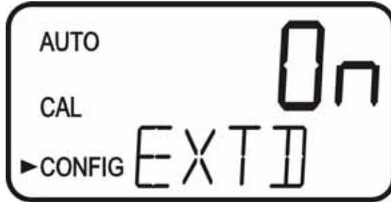
Press the  $\downarrow$  button a few times until the menus appear for **BITS**, **PRTY** (Parity) and **STOP** (Stop Bits). Set each one to the desired setting using the  $\uparrow$  and  $\downarrow$  buttons.
