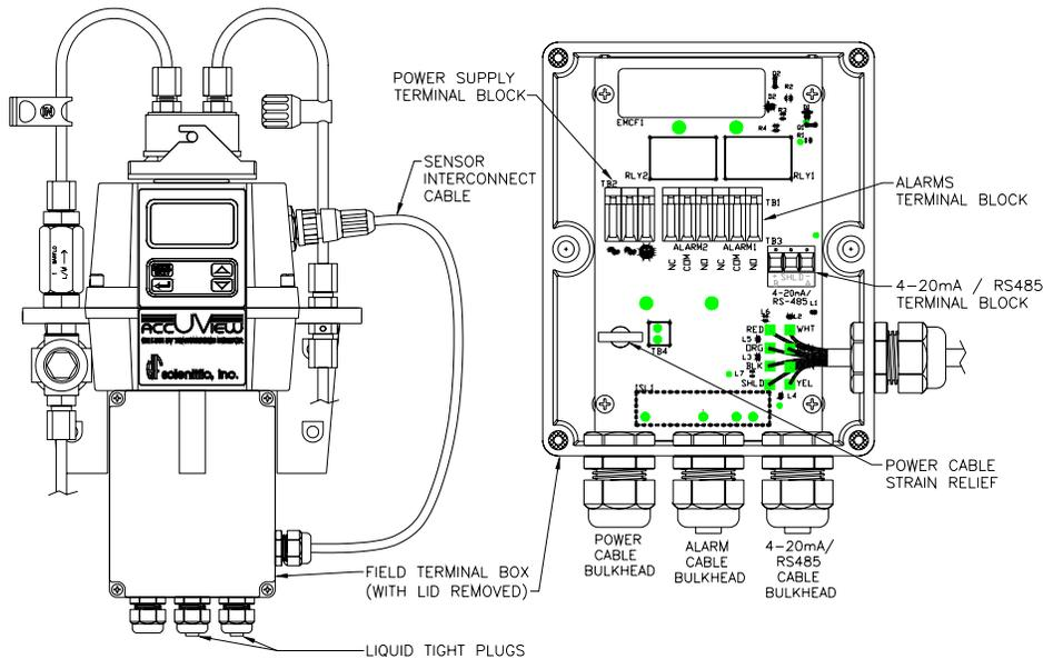
**Figure 1: Electrical Connections for the Instrument**
