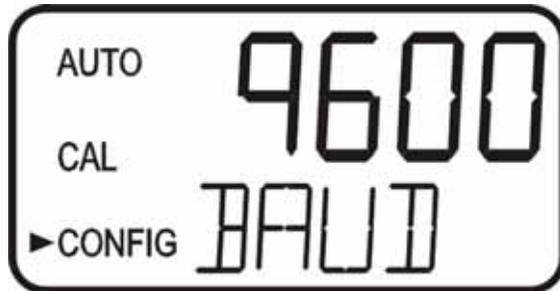
Press the **↵** button to continue on and select the desired instrument address (1-255) using the **▲** or **▼** buttons. Once the selection is satisfactory, press the **↵** button.
